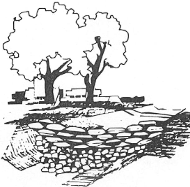
Sediment traps can be constructed in drainageways. Sandbags, straw bale barriers, and excavated sediment traps, placed at regular intervals within a drainage channel, are easy and economical to construct. Sandbag barrier sediment traps are constructed of bags filled with sand or crushed rock and stacked in an interlocking manner designed to trap sediment and reduce velocity of flow.
