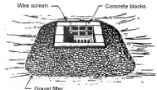
sediment pool. For slower drainage and therefore more settlement time, the concrete blocks could be eliminated and the device made entirely of gravel.
