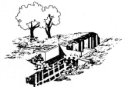
of flow, therefore, special care must be taken to prevent undercutting at the toe of the structure and erosion of the banks.
