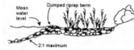
Reed berms, consisting of a combination of reeds and riprap, break wave action and erosion of banks by currents. Banks should not exceed a 2:1 slope. Riprap is placed to form a berm that extends beyond the surface at mean low-water level, separating the reed bed from the body of water.
